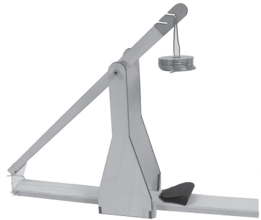
A Pitsco Trebuchet – the swinging weight absorbs much of the excess force.
