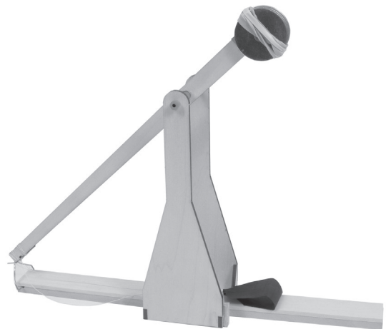
A trebuchet with a fixed weight and no wheels – the machine absorbs much of the force.
